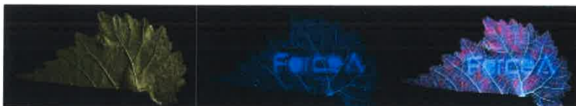
Three views of the same leaf. The FORCE-A logo has been drawn on a grapevine leaf by UV-C application, which induces the stilbenes, through a stencil. Fluorescence measurement under UV-A excitation.
