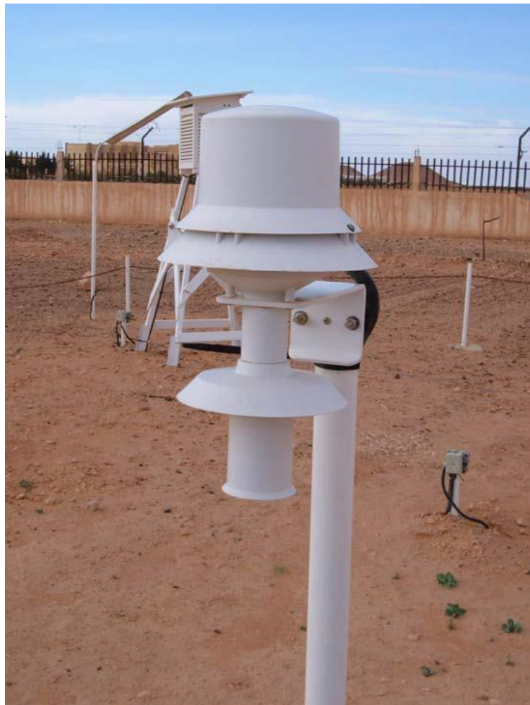
Figure 1. Example of shielded thermometer and hygrometer with forced ventilation (43502 YOUNG). Source WMO Field Intercomparison of Thermometer Screens and Humidity Measuring Instruments, Ghardaïa, 2008-2009, Appendix 1
