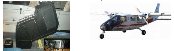
Figure 4. TASI-600 sensor mounted on the Partenavia P68 Observer airborne.
