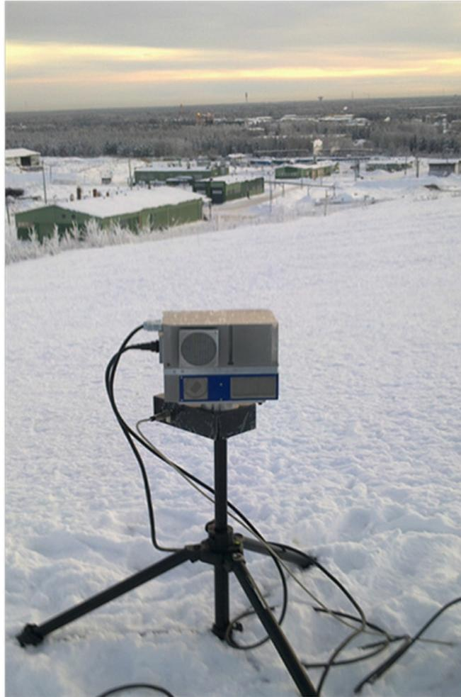
Figure 10. The cooled LWIR-C camera installed on a rotary stand for outdoor scanning.
