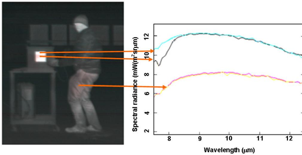
Figure 12. Outdoor methane gas detection experiment with methane flow rate of 20 l/min. Methane flow is visualized in reddish color in the scanned image. Methane absorption around 7.7  $\mu\text{m}$  is clearly seen in the radiance spectrum (black spectral plot) against the blackbody surface (cyan spectral plot).
