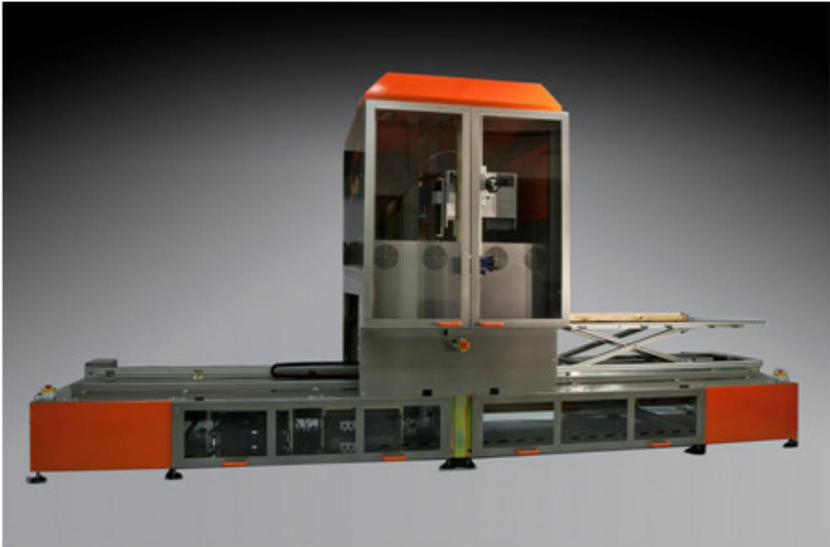
Figure 9. An industrial hyperspectral imaging scanner, SisuROCK, for rapid mineral mapping in drill cores and other geological samples.
