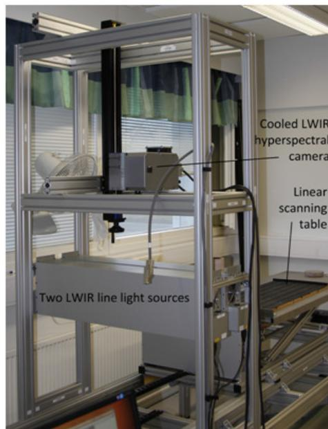
Figure 6. LWIR scanning setup for imaging experiments in reflectance mode
