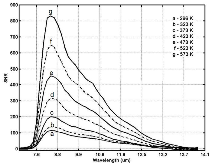
Figure 5. SNR in the uncooled spectral camera LWIR HS with different blackbody target temperatures (a to g).
