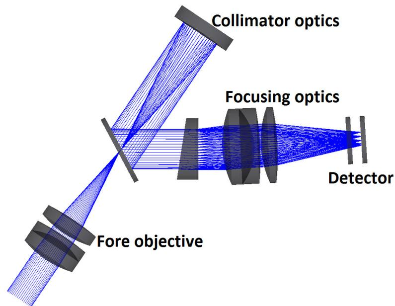
Figure 1. Schematic optical design of the imaging spectrograph in SPECIM's LWIR hyperspectral cameras. The diffracting element is before the focusing optics.
