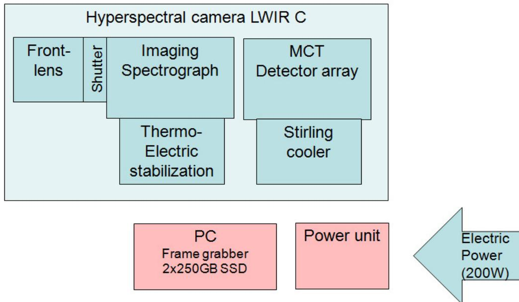
Figure 3. Block diagram of the cooled LWIR hyperspectral camera.
