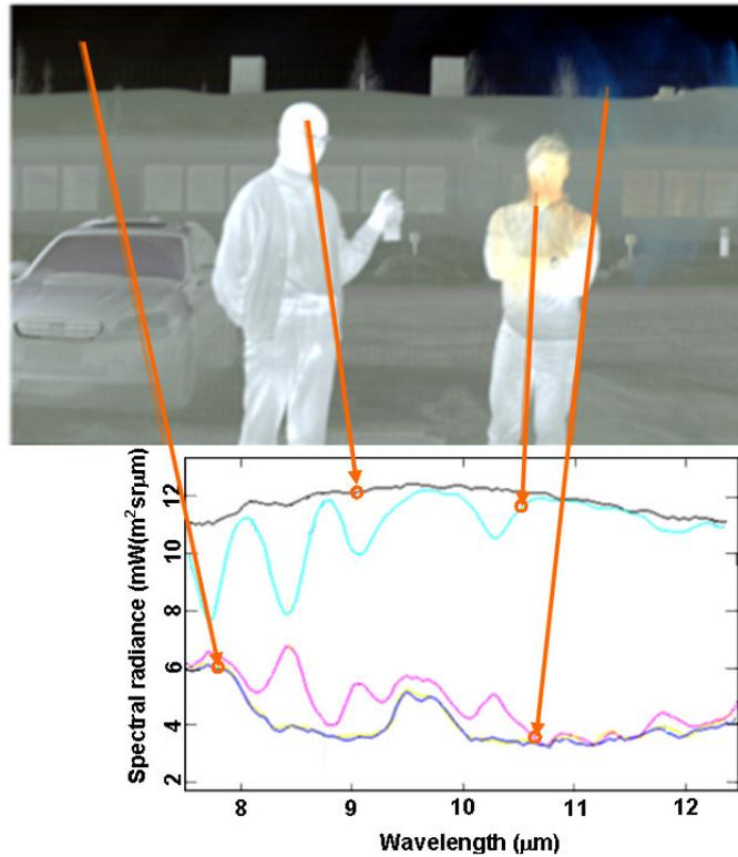
Figure 11. Outdoor gas measurement experiment with the cooled spectral camera LWIR-C in ambient temperature of -15 C. Propellant gas (1,1,1-2 tetrafluoroethane) is detected based both on its emission (magenta spectral plot) and absorption (cyan spectral plot).
