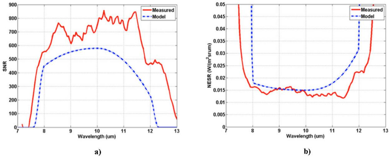
Figure 4. SNR (a) and NESR (b) in the cooled spectral camera LWIR C at the middle of the field of view as a function of wavelength. Both the simulated and measured curves are shown. The data has been averaged by two spectral pixels.
