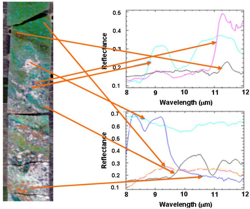
Figure 7. A piece of a classified drill core image which was scanned with the cooled LWIR spectral camera with 0.4 mm spatial resolution. Spectra on the top, cyan: clinopyroxene, black: carbonate, magenta: unknown mineral.
