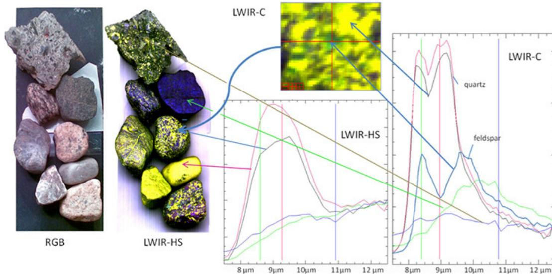
Figure 8. A set of stones were scanned with the uncooled LWI-HS and cooled LWIR-C spectral camera in reflection mode. The LWIR-C produces higher spectral resolution, leading to much more accurate mineral identification. In the zoomed LWIR-C image, the quartz and feldspar spectra are clearly recognizable.
